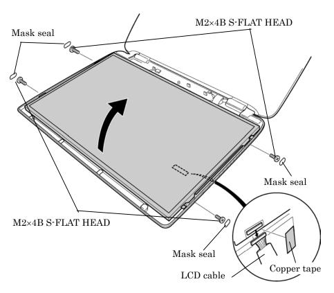
Figure 4-40 Removing the LCD module (1)
